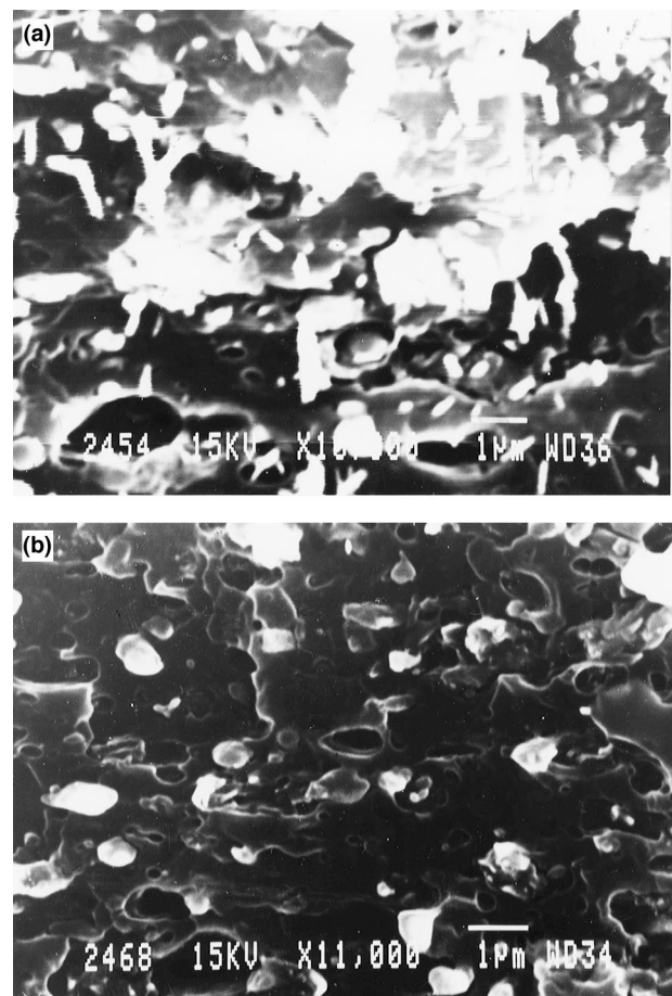
Fig. 14. SEM fractographs of (a) skin and (b) core sections of the injection-moulded PVC/5% LCP specimen.
